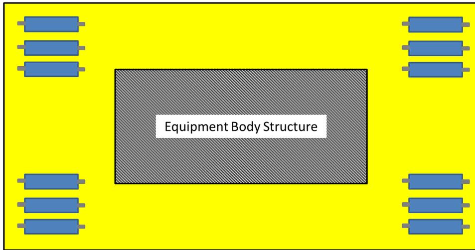
**Figure 3: Example Mudmat Anode Layout with Parallel Arrays (Not Preferred)**
