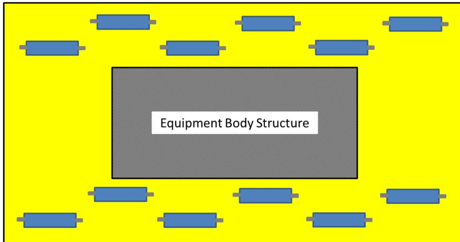
**Figure 6: Example Mudmat Anode Layout with Staggered Anodes (Preferred)**
