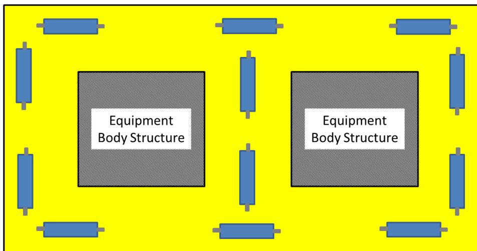
**Figure 5: Example Mudmat Anode Layout with Perpendicular Anodes (Preferred)**
