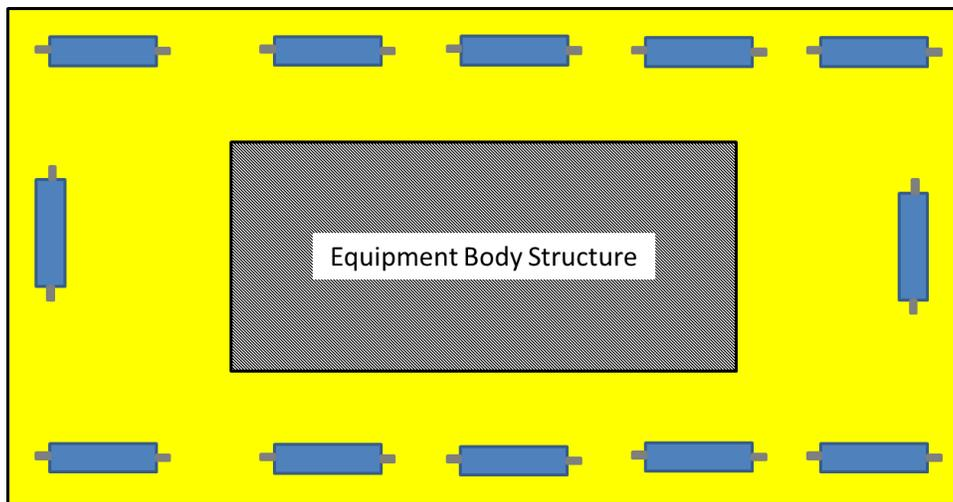
**Figure 4: Example Mudmat Anode Layout with End to End Anodes (Preferred)**
