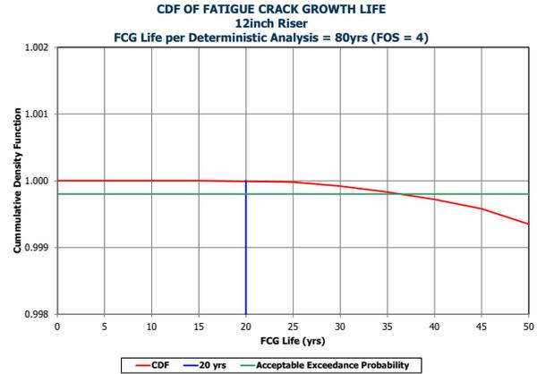
Figure A.2 - CDF Tail of FCG Life for 12inch Riser, Initial Flaw Size with 80yr Deterministic FCG Life
