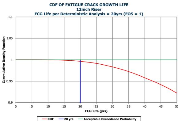
Figure A.1 - CDF Tail of FCG Life for 12inch Riser, Initial Flaw Size with 20yr Deterministic FCG Life
