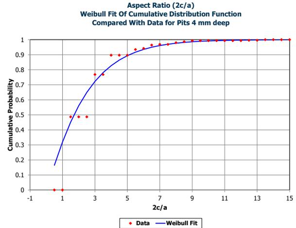
Figure 3 - Typical Distribution for Aspect Ratio for Pitting
