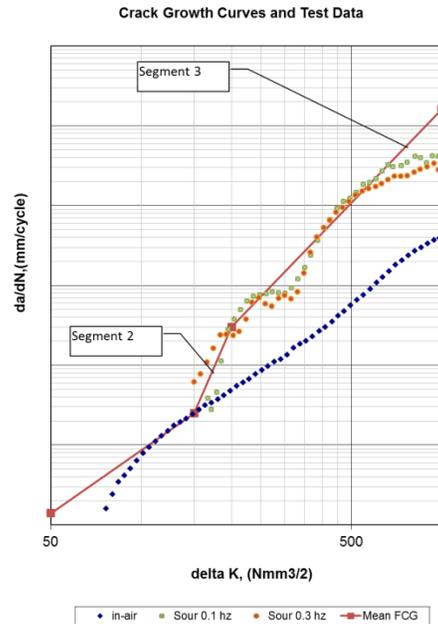
**Figure 4 – Characteristic Fatigue Crack Growth in Corrosive Environment**
