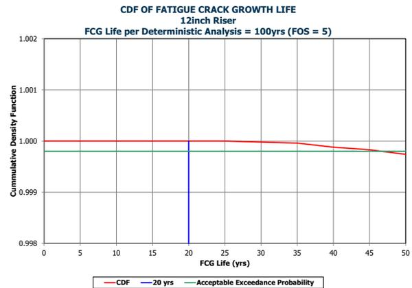
Figure A.3 - CDF Tail of FCG Life for 12inch Riser, Initial Flaw Size with 100yr Deterministic FCG Life
