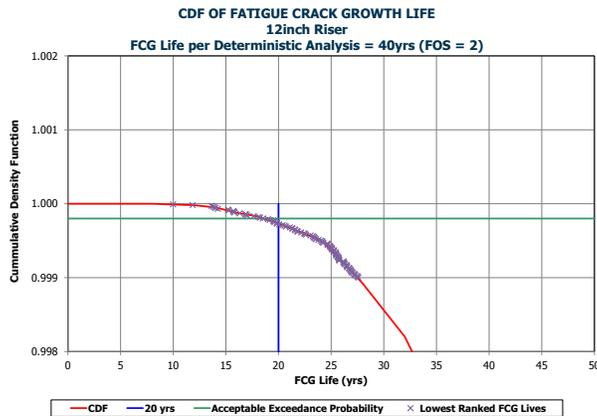
**Figure 8 – CDF Tail of FCG Life for 12inch Riser, Initial Flaw Size with 40yr Deterministic FCG Life**
