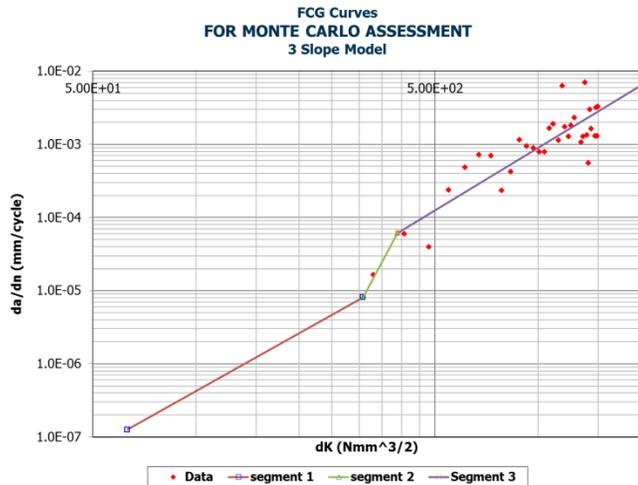
Figure 5 – Fatigue Crack Growth for Riser
