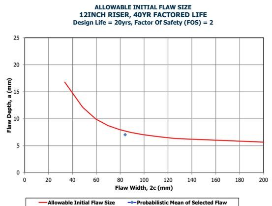
**Figure 7 – Allowable Initial Flaw Size, 40yr Factored Life, Factor of Safety = 2**
