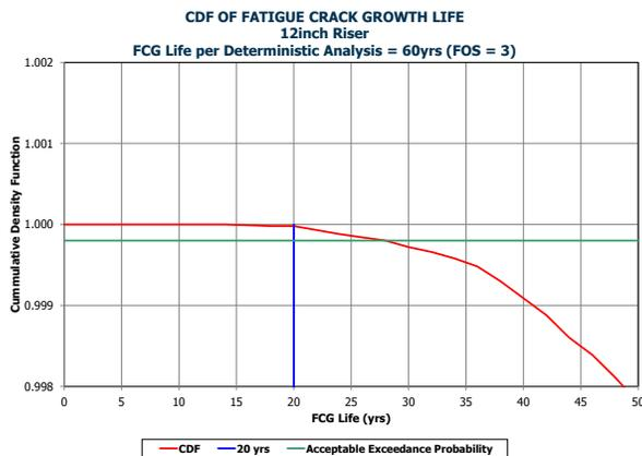
**Figure 9 – CDF Tail of FCG Life for 12inch Riser, Initial Flaw Size with 60yr Deterministic FCG Life Flowline**
