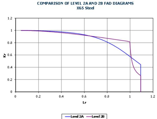
Figure 1 – Examples of FAD Diagrams for FFS Process.
