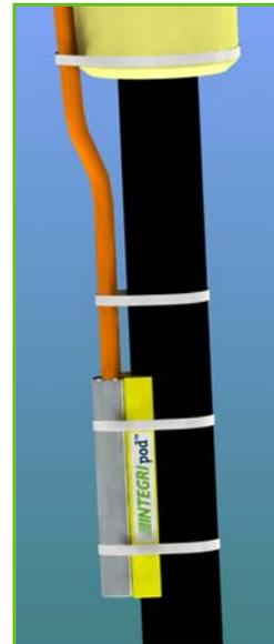
**Figure 16 – Left: View of flexASSURE Sensor in a Prototype Casing Installed Offshore.
