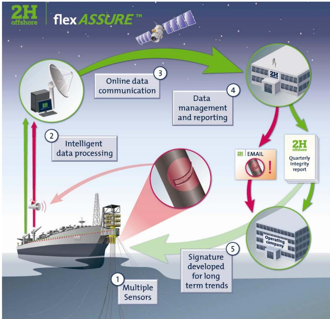
Figure 9 – flexASSURE™ Monitoring System Data Management Scheme
