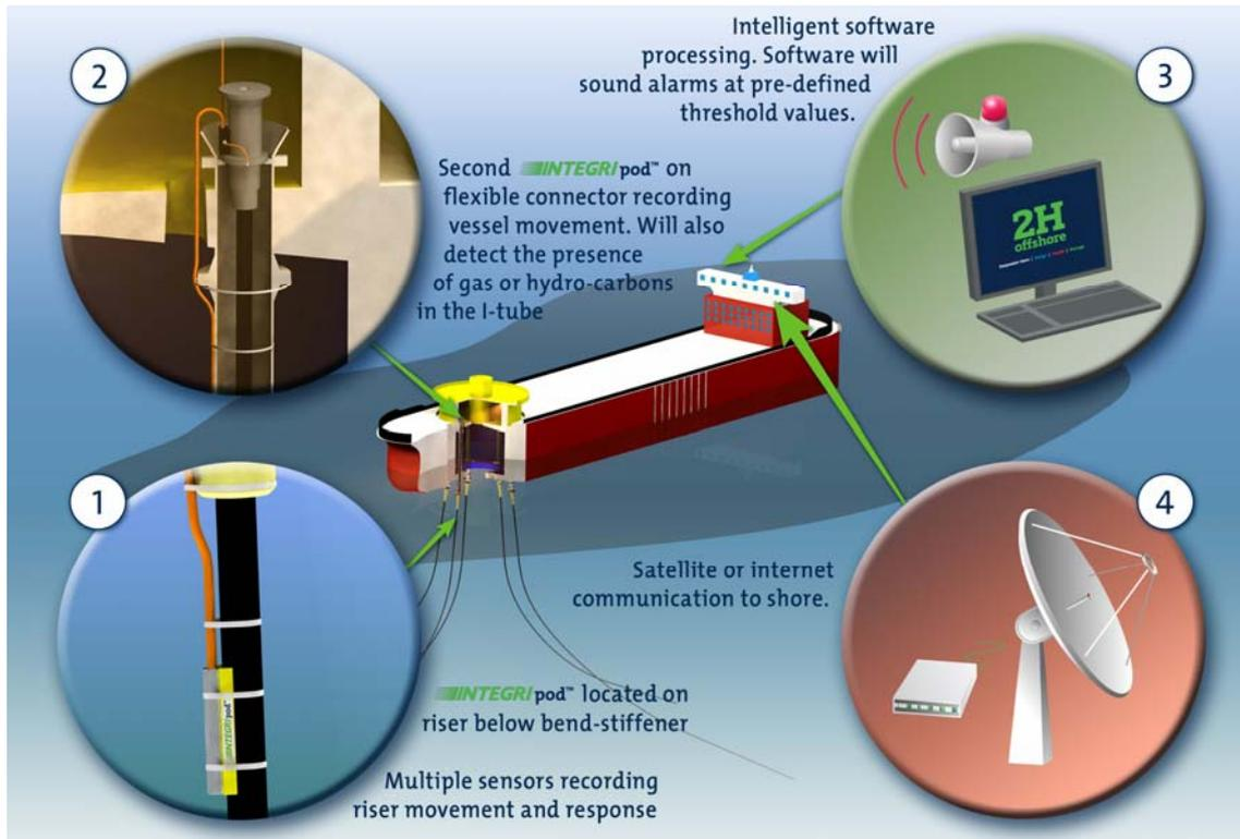
**Figure 8 – flexASSURE™ Monitoring System Components Overview**
