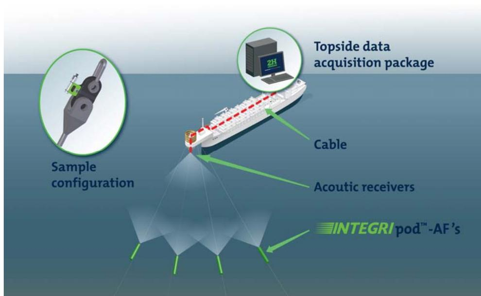
**Figure 7 – moorASSURE™ Monitoring System Schematic Description**
