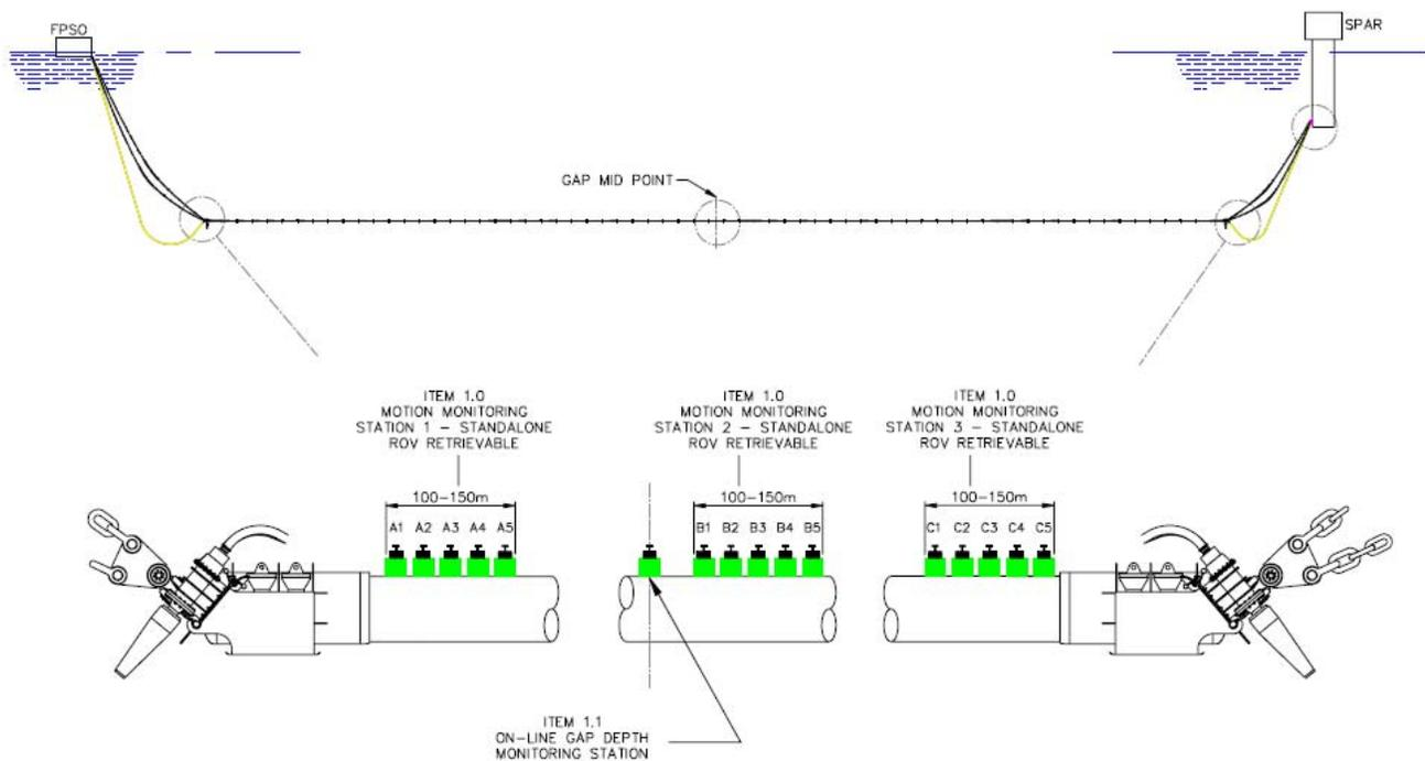
**Figure 3 – Bundled Mid-Water Flowline Monitoring System**
